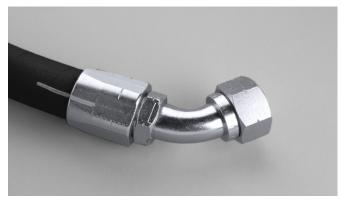
Once the hexagon of the fitting has contacted the socket, back off the fitting in order to align it correctly. The maximum permissible gap between the hexagon and the socket shoulder is 3mm
