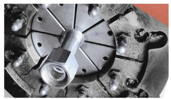
Ensure that the full length of the ferrule is covered by the dies
