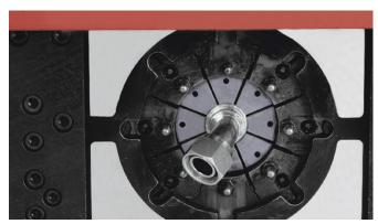
Ensure that the full length of the ferrule is covered by the dies
