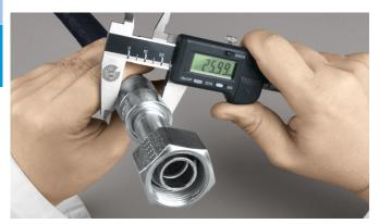
10 Inspect the crimped dimension using a calibrated vernier. Check the diameter at the centre of the ferrule against the relevant value in the latest version of the crimping data
