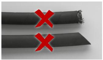
The end of the hose should be cut squarely to ±2° and there should be no ragged edges
