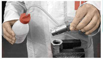
Secure the hose and socket vertically in the bench-vice. Using a suitable oil, generously lubricate the thread and taper of the fitting as well as the inside of the hose and socket.
