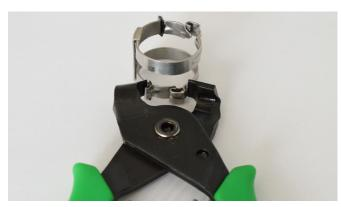
NOTE: Due to the size of the DN22 clamp it is necessary to compress it slightly by hand so that the pilers can fit over the clamping hooks
