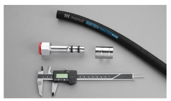
Check the dimensions of the components
