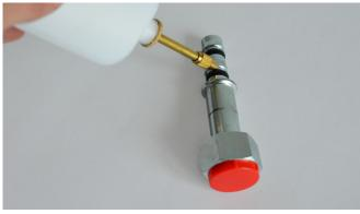
Grease the end of the fitting with the same oil used in the air conditioning system
