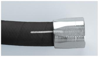
Use an indelible pen to mark the relative positions of the socket and the hose. This will make it easy to check that no unwanted rotation of the socket on the hose has occured.
