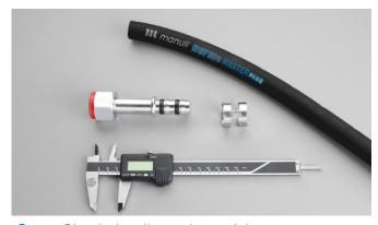
1 Check the dimensions of the components
