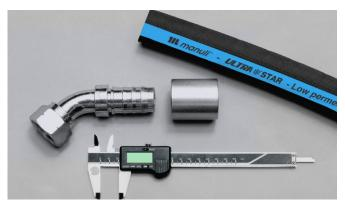
Check the dimensions of the components
