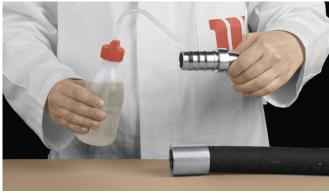
Grease the end of the fitting with the same oil used in the air conditioning system
