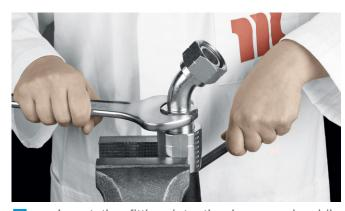
Insert the fitting into the hose and, while pressing down slightly, tighten it with a wrench by turning clockwise. Turn the fitting with a smooth, continuous motion to prevent damage to the hose.
