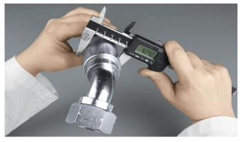
Inspect the crimped dimension using a calibrated vernier. Check the diameter at the centre of the ferrule against the relevant value in the latest version of the crimping data
