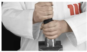
Secure the socket vertically in a bench-vice and screw in the hose, turning counter-clockwise, until it reaches the bottom of the socket. Unscrew the hose by ¼ turn to prevent damage in later steps.
