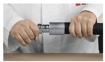
Fully insert the fitting into the hose and rotate the fitting to be in the correct orientation
