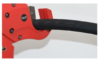
2 Cut the end of the hose using the manual cutter
