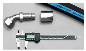
Check the dimensions of the components
