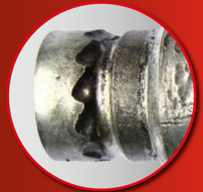
Brinelling on the male coupling
