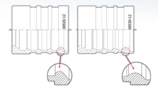
In particular, the improved geometry of the last tooth (*shown above*) has been proven to be highly effective at preventing wire breakage, whilst ensuring a robust grip on the hose reinforcement. This change has resulted in the new ferrule becoming approximately 2mm longer, however this does **not affect crimping parameters**, which will remain the same as listed for M00920-12 in the current publication of the **Crimping Booklet (March 2020 Edition)**.
