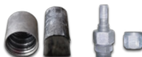
E-Coat 1000 after 1,000 hours ASTM B117 (ISO 9227) salt spray test
