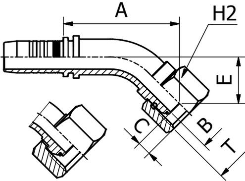
**45° BSP O-RING FEMALE SWEEP ELBOW 60° CONE
