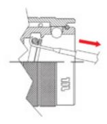
Remove the damaged O-ring and back-up ring.
