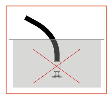
The Manuli hydraulic hose product range is not designed for immersion in the service fluid. This type of special application should be avoided or carefully studied with reference to the hose specifications
