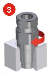
Use a wrench on the lower hexagon to tighten the new coupling to the torque listed below
