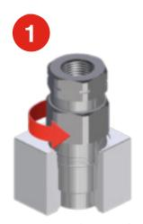
Use a wrench on the lower hexagon to unscrew the old coupling
