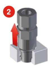
Lift out the old coupling and replace with the new part
