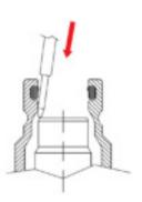
Use a suitable tool to pull back the valve and hold it in place.
