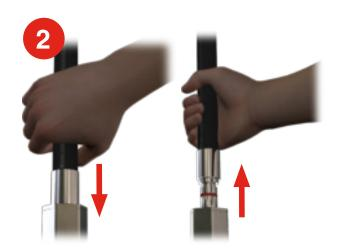
Push the fitting in until the collar touches the cartridge, then pull out to complete the disconnection process. Use a flat-headed screwdriver, or similar tool, to remove the protective cap on the cartridge.
