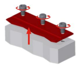
Unscrew the fixing screws and remove the old cover.
