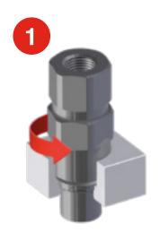
Use a wrench on the lower hexagon to unscrew the old coupling
