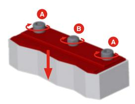
Place the new cover on the face of the fixed part and insert the screws into the positions shown.
